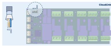
7 Check that the RS485 wire is the correct twisted pair + 1 and shield. FuelCloud recommends the Belden 8106A:
