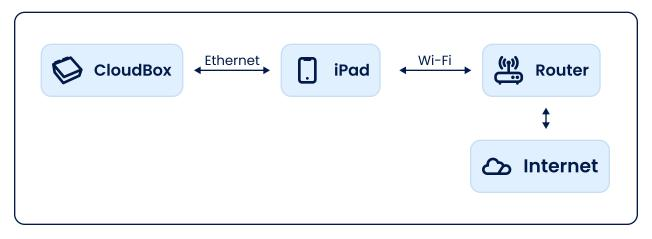
If cellular and hardwired ethernet are not options for connecting the iPad to the internet, the iPad can be connected to a Wi-Fi network. You will need to enter both the SSID and the password to bring the iPad online. The CloudBox can be connected directly to the iPad through ethernet.
