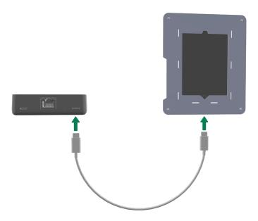
8 Connect an ethernet cable from the ethernet adapter to the CloudBox or to a router/switch.
