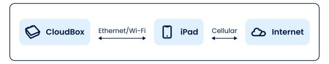
The iPad can communicate with the internet through cellular. The iPad will then communicate with the CloudBox over Wi-Fi or ethernet. FuelCloud recommends connecting the iPad directly to the CloudBox with the included ethernet cable.
