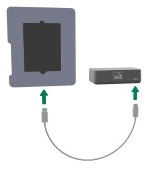
**4** Connect an ethernet cable from the PoE injector to the CloudBox or to a router/switch.
