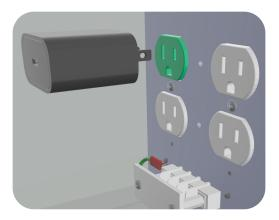
2 Connect the USB-C cable from the iPad power adapter to the ethernet adapter.
