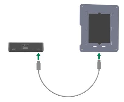
4 Connect an ethernet cable from the ethernet adapter to the CloudBox or to a router/switch.
