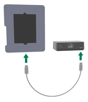
**4** Connect an Ethernet cable into the Ethernet adapter and then connect the other end of the Ethernet cable into the CloudBox or into a router/switch.
